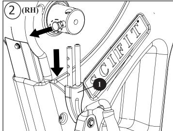
Position the curvature of the crank in the same direction as the left side crank.
