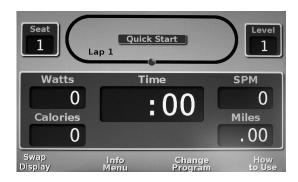
This program automatically starts just by moving the arm handles or foot pedals. It also bypasses entering goal information. The user can manually change the workload as desired by using the up and down arrow buttons.
