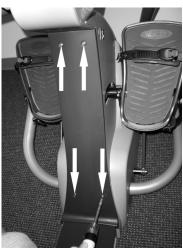
3. Remove 2 screws from right upper cover and remove cover from frame.
