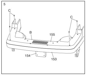
With the help of a second person, set the Handrail Base (154) on the Uprights (149, 150).
