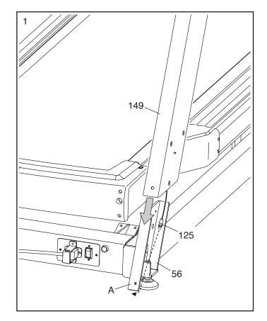
Partially tighten four 5/16" x 3/4" Screws (51) with three 5/16" Star Washers (61) into the Left Upright (149) as shown; do not fully tighten the Screws yet.
