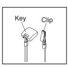
console, causing the walking belt to slow to a stop. Test the clip by carefully taking a few steps backward; if the key is not pulled from the console, adjust the position of the clip.
