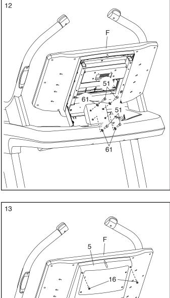
Attach the Console Back (5) to the console assembly (F) with four #8 x 3/4" Screws (16); start all four Screws, and then tighten them. Do not overtighten the Screws.
