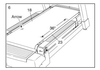
Next, move the Walking Belt (18), if necessary, until the seam (not shown) across the Walking Belt is beneath the Walking Platform (23).
