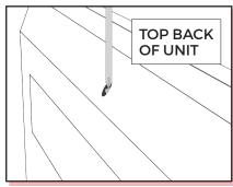
2. Using a Philips screwdriver, drive in the screw located above wall mount to secure.
