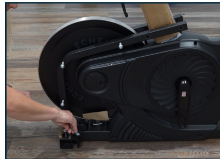
Remove bolts on both sides with included tool as shown.
